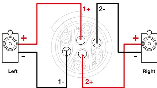
**Bridge-Tied Load Wiring**
